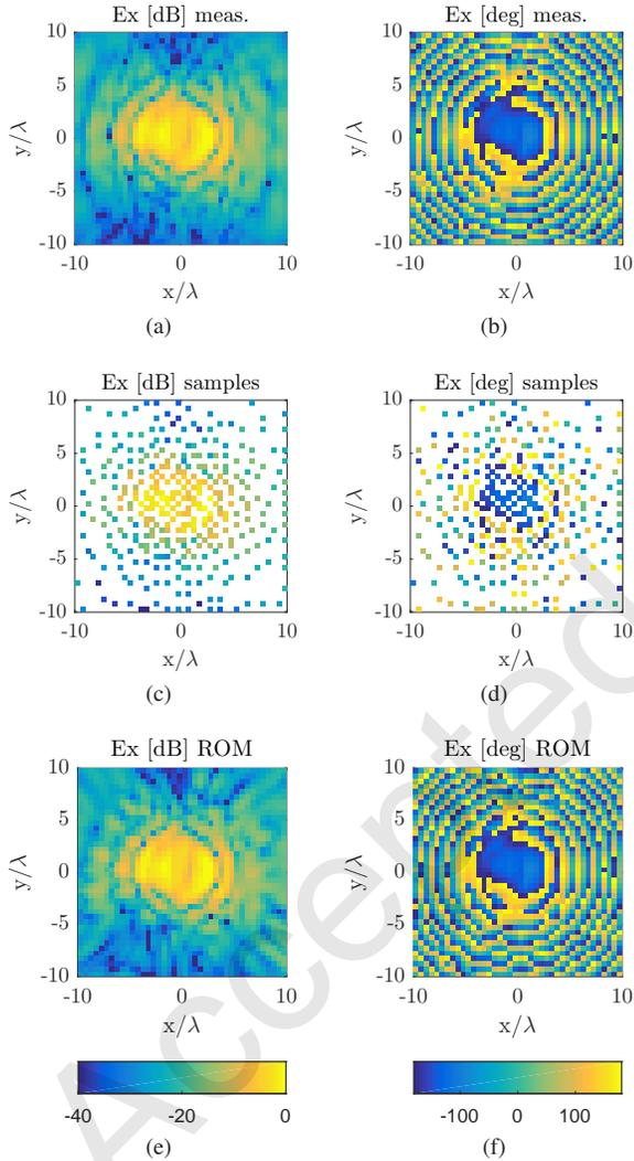
Fig. 6: Planar near field mappings (left (a,c,e) magnitude and right (b,d,f) phase) radiated by the metasurface at 32 GHz at a height of  $5\lambda$ . Near field mappings of (top (a,b)) the measured data, (middle (c,d)) the samples selected by the DEIM and (bottom (e,f)) the reconstructed field using the ROM approach.
