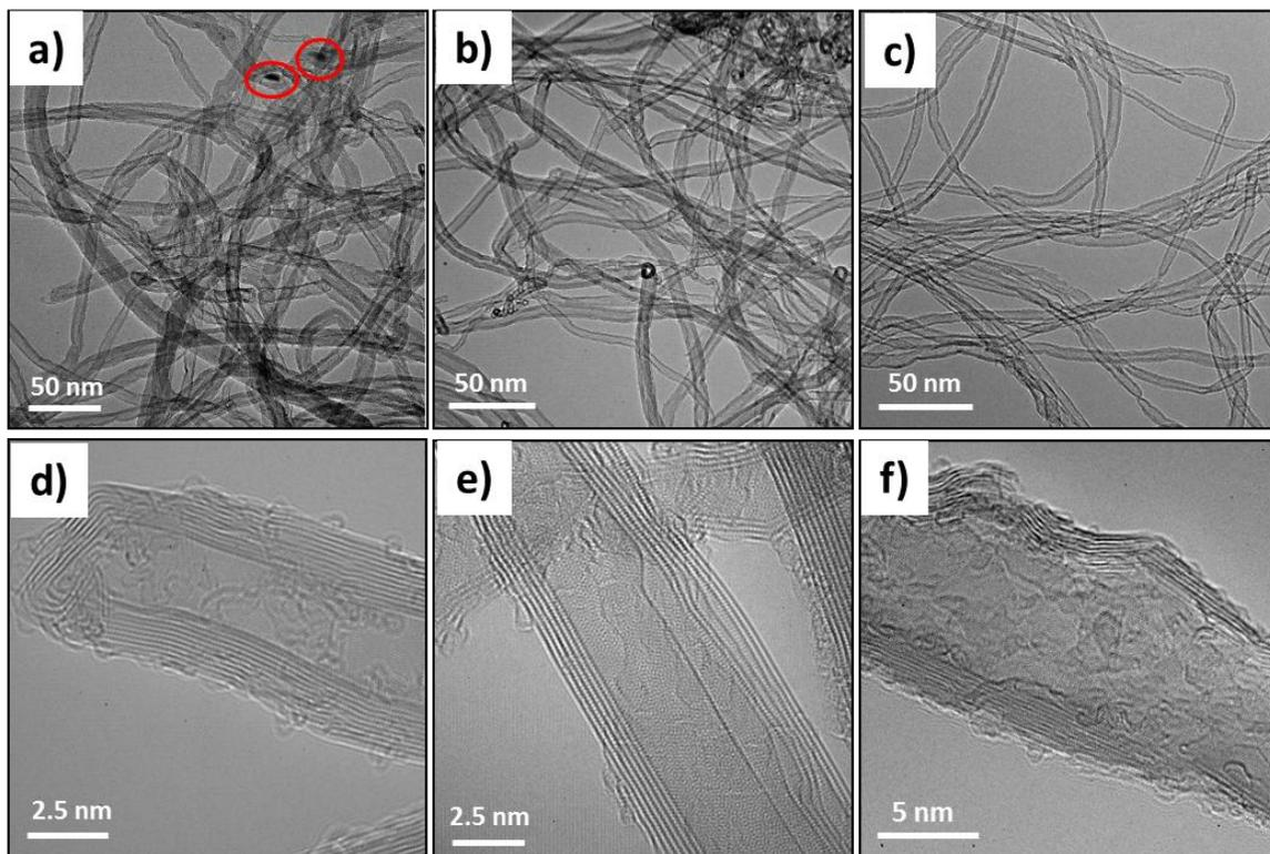
**Figure 2.** Typical TEM bright field micrographs of the MWCNT samples. a) and d) r-MWCNT; b) and e) p-MWCNT; c) and f) f-MWCNT at different magnifications.
