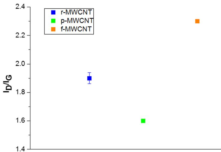
**Figure 3.** I<sub>D</sub>/I<sub>G</sub> ratios of r-MWCNT (blue), p-MWCNT (green) and f-MWCNT (orange). The error bars were determined from the standard deviation to the calculated ID/IG average.
