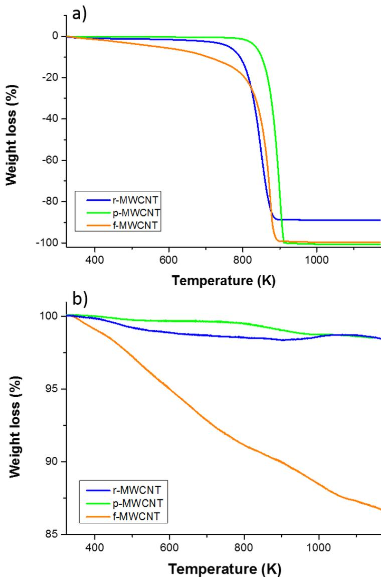
**Figure 1.** Thermograms recorded of r-MWCNT (blue curve), p-MWCNT (green curve), f-MWCNT (orange curve); a) in dry air and b) in helium.
