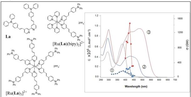
Figure 2. Left : Chemical structures of La,  $[Ru(La)(bipy)_2]^{2+}$ ,  $[Ru(La)_3]^{2+}$ . Right: 1PA and 2PA spectra for La (dotted curves;  $\mathcal{D}$ ),  $[Ru(La)(bipy)_2]^{2+}$ (blue curves;  $\mathcal{Q}$ ),  $[Ru(La)_3]^{2+}$ (red curves;  $\mathcal{Q}$ ), in  $CH_2Cl_2$  (10<sup>-6</sup> M).
