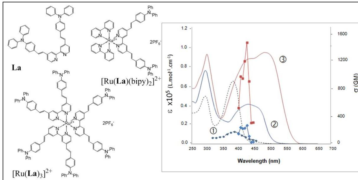
Figure 2. Left: Chemical structures of **La**,  $[\text{Ru}(\text{La})(\text{bipy})_2]^{2+}$ ,  $[\text{Ru}(\text{La})_3]^{2+}$ . Right: 1PA and 2PA spectra for **La** (dotted curves; ①),  $[\text{Ru}(\text{La})(\text{bipy})_2]^{2+}$  (blue curves; ②),  $[\text{Ru}(\text{La})_3]^{2+}$  (red curves; ③), in  $\text{CH}_2\text{Cl}_2$  ( $10^{-6}$  M).
