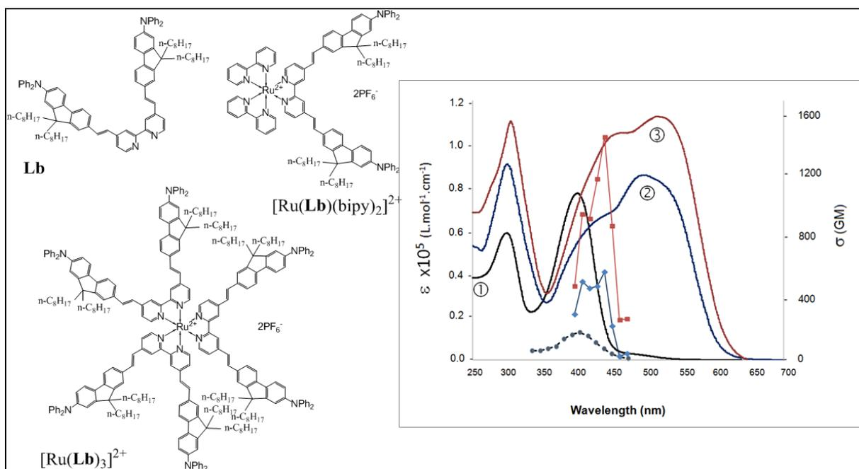
Figure 3. Left : Chemical structures of **Lb**,  $[\text{Ru}(\text{Lb})(\text{bipy})_2]^{2+}$ ,  $[\text{Ru}(\text{Lb})_3]^{2+}$ . Right: IPA and 2PA spectra for **Lb** (black curves; ①),  $[\text{Ru}(\text{Lb})(\text{bipy})_2]^{2+}$  (blue curves; ②),  $[\text{Ru}(\text{Lb})_3]^{2+}$  (red curves; ③), in  $\text{CH}_2\text{Cl}_2$  ( $10^{-6}$  M).
