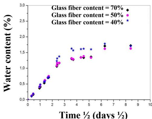
Figure 3: Water content for different glass fiber contents
