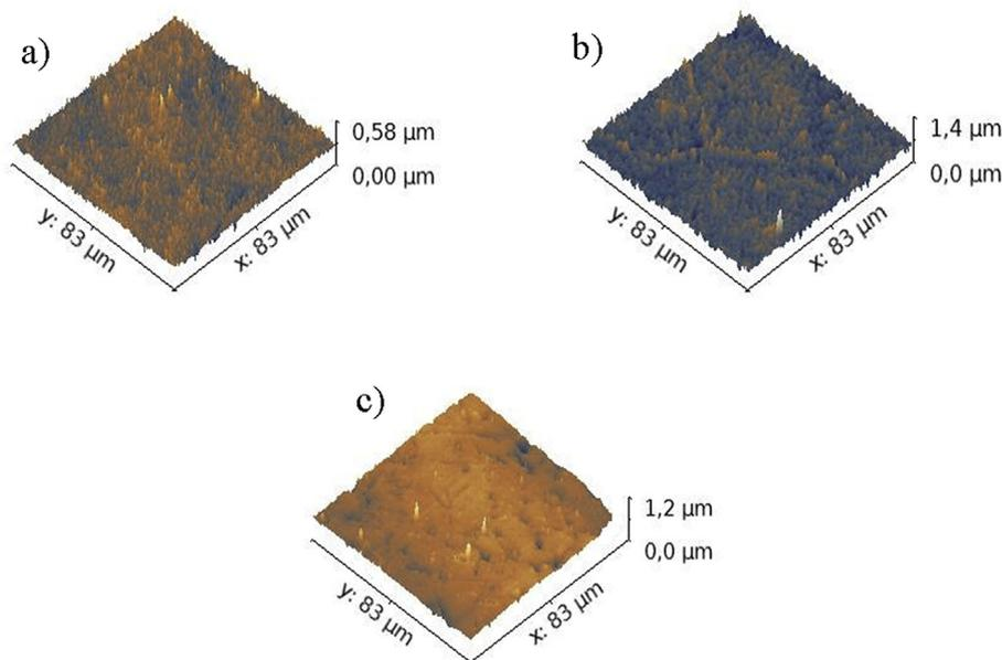
Fig. 3. AFM surface scans from: a) bare Ti–27Nb; b) nitrided Ti–27Nb; c) NiTi, alloy.
