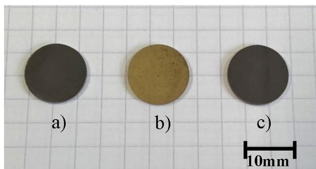
Fig. 1. Visual appearance of a) bare Ti-27Nb, nitrided Ti-27Nb, c) NiTi, alloy.
