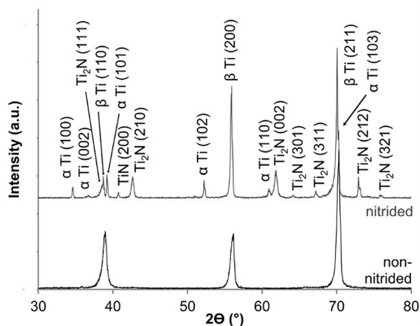
Fig. 2. XRD patterns of nitrided and non-nitrided Ti-27Nb alloy.
