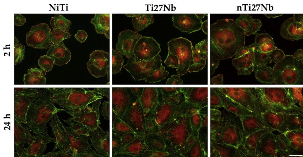
Fig. 4. Fluorescent microscopy images of EPC cells cultured for 2 h and 24 h on NiTi, bare Ti–27Nb and nitrided Ti–27Nb (nTi27Nb) surfaces. Actin microfilaments and vinculin are stained green and red. Scale bar represents 50 μm. (For interpretation of the references to color in this figure legend, the reader is referred to the Web version of this article.)
