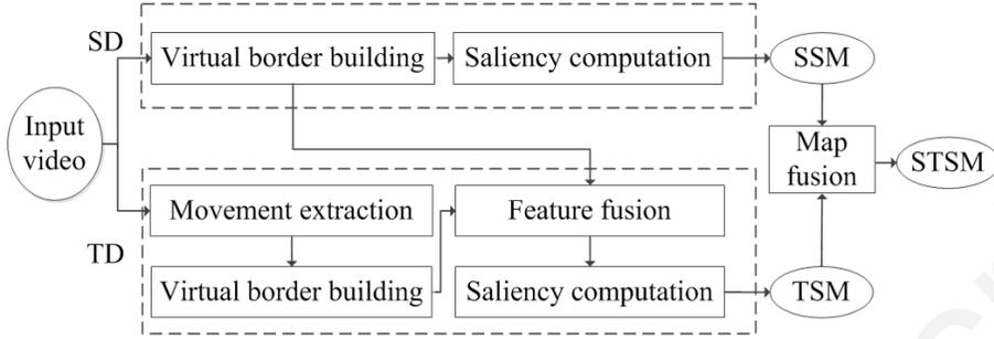
Figure 3: The proposed block-diagram. SD: spatial saliency detection; SSM: spatial saliency map; TD: temporal saliency detection; TSM: temporal saliency map; STSM: spatio-temporal saliency map.
