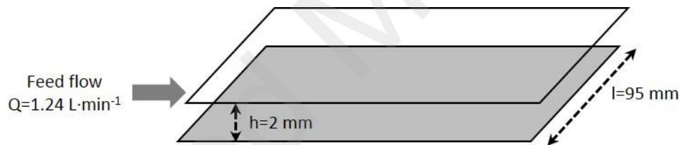
**Figure 6.** Outline of the inside of the SEPA cell
