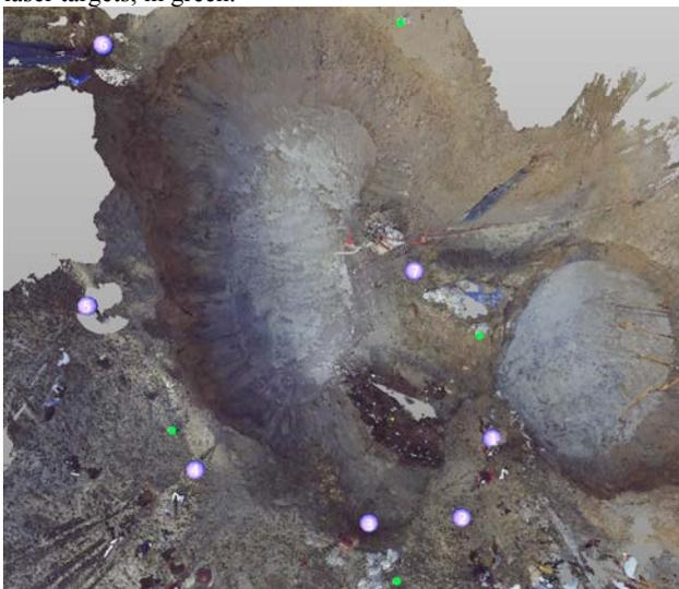
Figure 11. Laser scanner and targets positions
