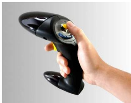
Figure 16. The Flystick 2 device
