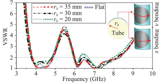
Fig. 7. Measured VSWR of the antenna under various  $x$ -axis (thin lines) and  $y$ -axis (thick lines) bending radii compared to that of the flat case (triangle symbol). The inset illustrates the bending test scenarios over plastic tube.
