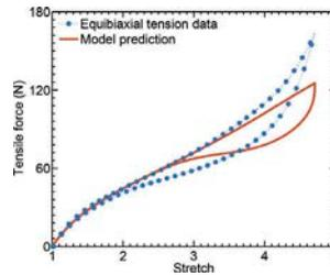
Figure 4. Comparison between model predictions and experimental data of natural rubber in equibiaxial tension.
