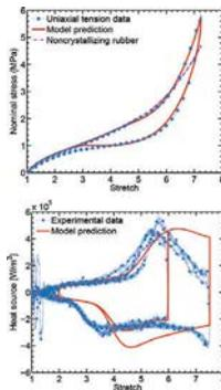
Figure 3. Predictions of the proposed model in the case of strain-induced crystallization in comparison to experimental data of natural rubber undergoing uniaxial tension: stress-stretch response (top), and evolution of heat source (bottom).
