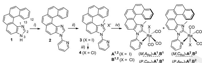
**Scheme 1.** Synthetic access to helicene-NHC-Re complexes **A** and **B**. i) 2-Br-pyridine, K<sub>2</sub>CO<sub>3</sub>, CuI (cat.), L-Pro (cat.), DMSO, 110°C, 63 h; 69%; ii) MeI, MeCN, reflux, overnight; 83% (2 steps); iii) Dowex resin, acetone; 88%; iv) ReCl(CO)<sub>5</sub>, K<sub>2</sub>CO<sub>3</sub>, toluene, reflux, 22 h; 65% (**A**<sup>1,2</sup>), 54% (**B**<sup>1,2</sup>).
