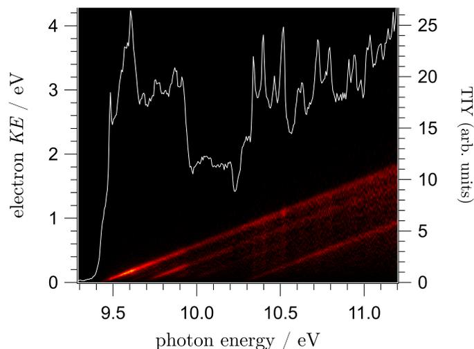
Fig. 2 Mass-selected photoelectron signal as a function of the photon energy (horizontal axis) and electron kinetic energy (vertical axis), for  $m/q = 40$  a.m.u.. The corresponding total ion yield obtained by integrating over all electron kinetic energies is superimposed on the map as a white line.
