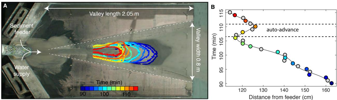
Figure 3: A) General setup seen from above and position of the coarse grain delta, and B) trajectory of the coarse-grain delta front between 90 (dark blue) and 124 min (red). Colored dots correspond to the delta front position mapped on panel A.
