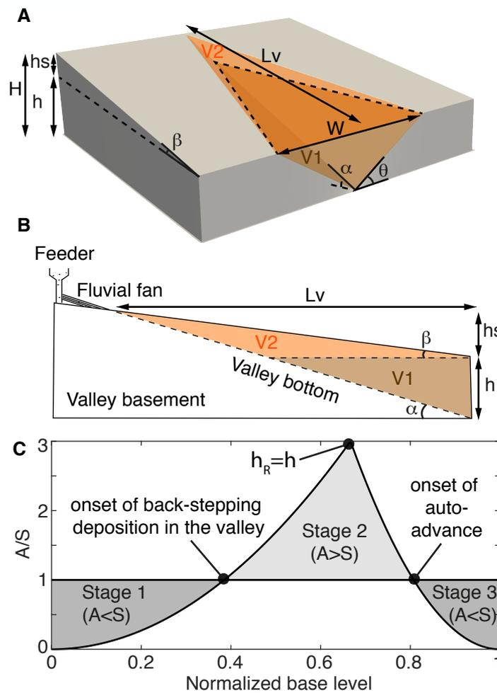
Figure 2: A) 3D schematic and B) cross-section views of an incised valley of height  $H$  (with  $h$  the elevation at slope break and  $h_s$  the height between the slope break and the valley apex), length  $L_v$ , width  $W$ , valley slope  $\alpha$ , valley side slope  $\theta$  and interfluve
