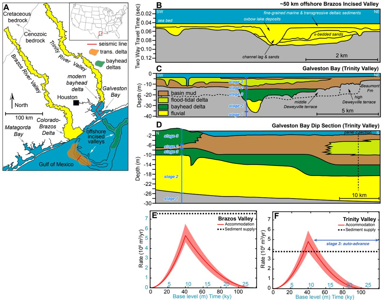
Figure 4. A) Study area in Texas Gulf of Mexico coast, B) cross-section of the Brazos River Valley, C) and D) cross- and dip- sections of the Trinity River Valley (modified from Simms et al., 2006; Anderson et al., 2008) showing the possible stages defined from our model. Locations of the sections are indicated on panel A (red). E) and F) Model outputs for the Brazos and Trinity systems, respectively, with the auto-advance time window for the Trinity indicated.
