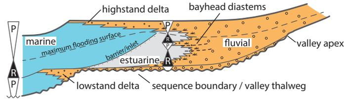
Figure 1. Incised-valley fill model with bayhead diastems and out-of-sequence bay-head progradation at the end of retrogradation (from Zaitlin et al., 1994). P: progradation, R: retrogradation.
