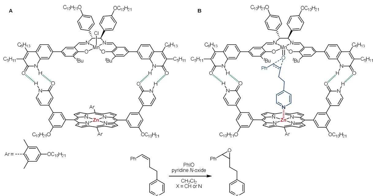
**Figure 4.** Warnmark's zinc(II)-porphyrin-based dynamic supramolecular manganese catalysts featuring substrate selectivity in epoxidation reactions *via* remote Zn $\cdots$ N interactions between the catalyst and the substrate (**A**) and the corresponding postulated transition state (**B**). Green dashed lines indicate intermolecular hydrogen bonding.
