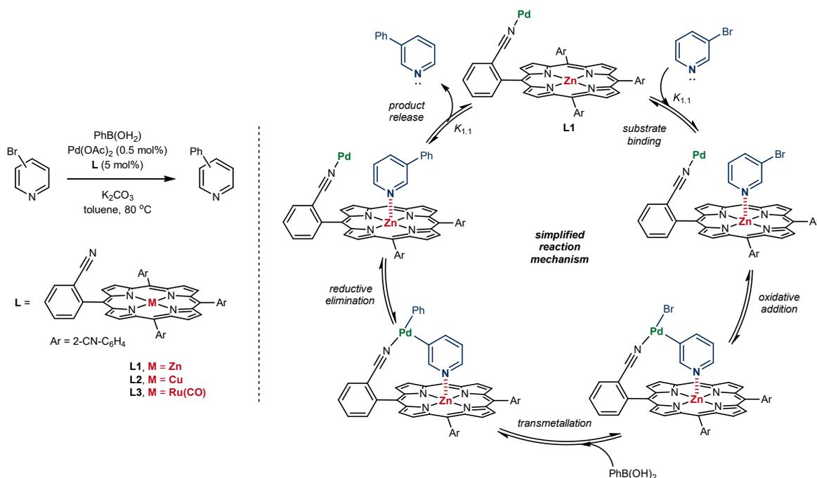
**Figure 6.** A supramolecular catalyst with a catalytically active palladium site and a substrate recognition site enabling  $\text{Zn}\cdots\text{N}$  interactions between substrate and catalyst, together with the postulated catalytic cycle.
